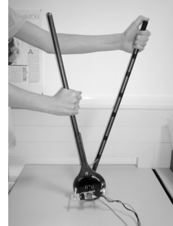
Figure 4. The DAMPER in the "edge-trimmer" configuration.
