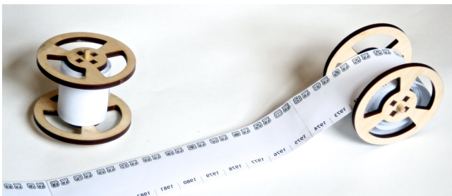
Figure 1. ChronoTape on spools. The spools act as both storage and a way of controlling the timeline when on the reader.
