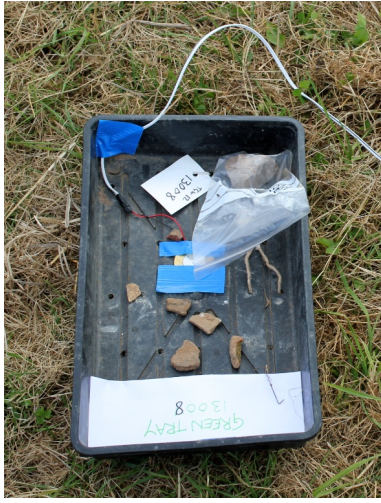
Figure 2 A 'Finds Tray' is used to store new items; each tray is connected to the ChronoTable. The activity level in each tray is measured with the piezoelectric sensor that detects vibrations in and around the tray.
