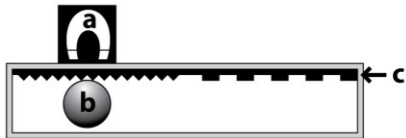
Figure 4. Experimental setup showing (a) magnet, (b) ball-bearing and (c) textures.
